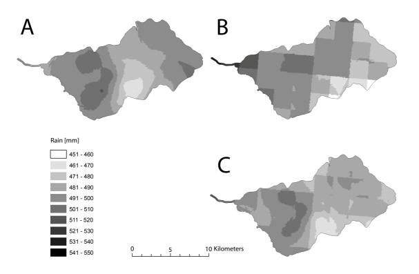
**Fig. 4.** Spatial distribution of total rainfall from March to October 2004 as derived by **(A)** ordinary kriging (mean value 492 mm), **(B)** operational available radar (mean value 490 mm) and **(C)** ordinary colocated cokriging (mean value 487 mm).
