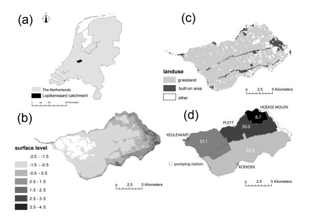
**Fig. 1.** (a) Location of Lopikerwaard catchment within The Netherlands; (b) Surface level of the Lopikerwaard catchment in meters + N.A.P. (reference sea level); (c) Land use in the Lopikerwaard catchment; (d) Subcatchments within the Lopikerwaard catchment with the corresponding pumping stations, area-size of each subcatchment is given in square kilometers.
