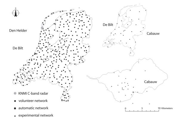
**Fig. 2.** Locations of raingauges and weather radars in The Netherlands; volunteer network with 330 raingauges (temporal resolution of 1 day), automatic network with 35 tipping bucket raingauges (temporal resolution of 10 min), experimental network with 30 tipping bucket raingauges (equipped with event loggers) and 2 C-band Doppler radars.
