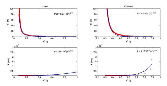
**Fig. 6.** Hillslope/REW scale soil hydraulic functions derived from simulated drainage experiments for a homogeneous hillslope with a loess soil (left panels, REV scale hydraulic parameters given in Table 1) and a homogeneous hillslope with a Colluvisol soil (right panels). The 95%-confidence limits as well as the  $R^2$  of the fits are given in Table 2.
