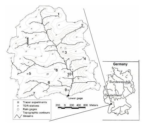
**Fig. 1.** Observational network of the Weiherbach catchment. Soil moisture was measured at 61 TDR stations at weekly intervals (crosses). Triangle indicates the stream gage. Topographic contour interval is 10 m.
