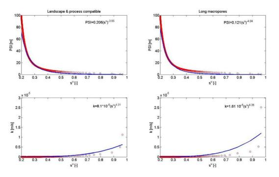
**Fig. 5.** Hillslope/REW scale soil hydraulic functions derived from simulated drainage experiments for the landscape and process compatible hillslope (left panels) and a hillslope with same spatial pattern of soils and macropores, but where the macropores reach continuously to the lower boundary of the modelling domain (right panels). The 95%-confidence limits as well as the  $R^2$  of the fits are given in Table 2.
