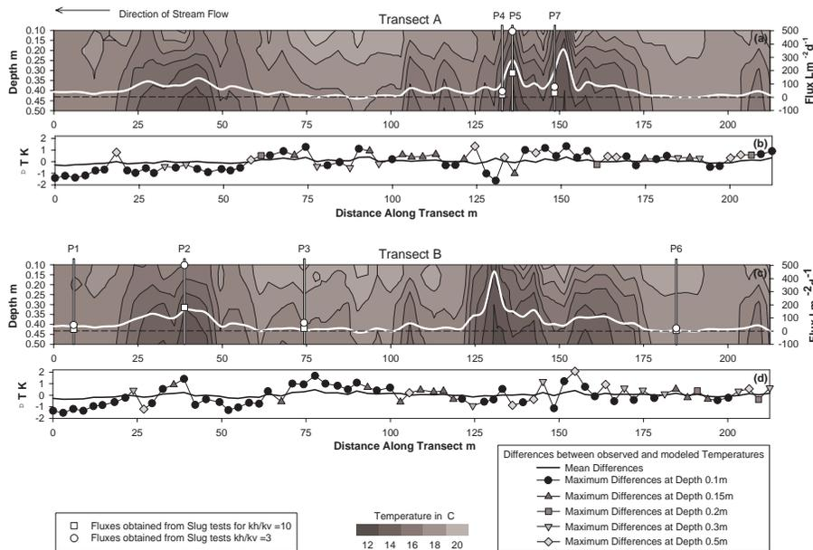
**Fig. 4.** Temperature distribution and temperature based fluxes and the locations of streambed piezometers and the fluxes from Darcy’s law calculations at each piezometer for different anisotropy ratios along Transects A (a) and B (c):
