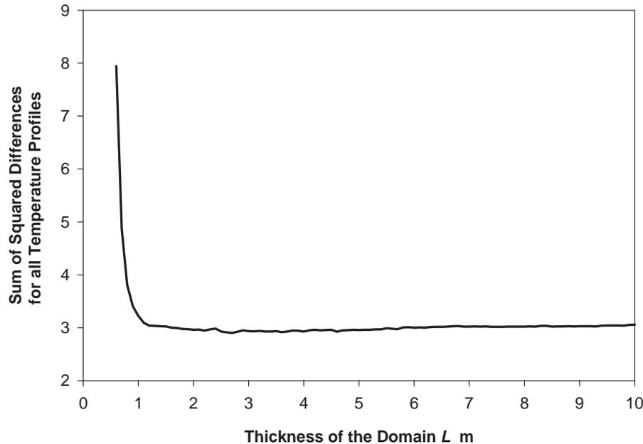
**Fig. 5.** Sum of squared errors of all temperature profiles vs. the length of the domain  $L$ . The results show that for the given parameter set, the quality of fit and the derived vertical fluxes are essentially constant for  $L > 1.0$  m.
