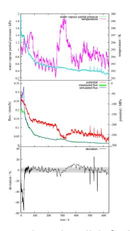
Fig. 11. Results of the evaporation experiment with the Grenzhof soil sample. that measured and simulated flux (middle frame) practically overlap. The relative deviation  $(j_{\text{exp}}^{w}-j_{\text{model}}^{w})/j_{\text{exp}}^{w}$  is shown in the bottom frame together with the measuring uncertainty from Fig. 13 (gray band).
