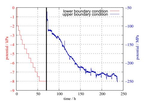
**Fig. 8.** Boundary conditions during the experiment with the sand sample. The red line shows the lower boundary condition during the MSO, the blue line the upper boundary condition during the evaporation experiment. A no-flow boundary condition was set at the upper boundary during MSO and at the lower boundary during evaporation. The black vertical line marks the switch between MSO and evaporation.
