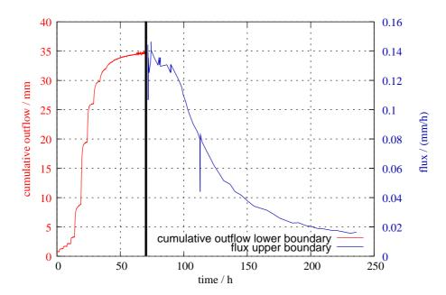
**Fig. 7.** Measured outflow of the sand sample. The red line shows the cumulative outflow at the lower boundary during MSO, the blue line the flux rate at the upper boundary during the evaporation experiment. The black vertical line marks the switch between MSO and evaporation.
