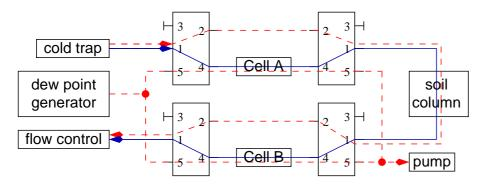
**Fig. 5.** Setup for runtime calibration. In normal operation (blue line), all valves are in state (1). During calibration (red dashed lines), the four valves are set to state (2), the measured gas bypasses the gas analyser and conditioned air from the dew point generator is flowing through both cells.
