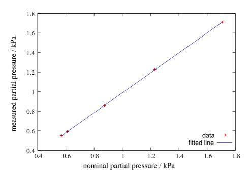
**Fig. 4.** Linearity and calibration check of the gas analyser. Null gas was flowing through cell A and air with defined water vapour molar fraction through cell B. The nominal cell B molar fraction was varied and the measured partial pressure  $\rho_{\rm meas}$  recorded.
