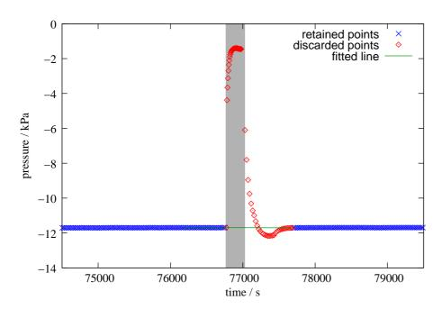
**Fig. 6.** Filtered data of the pressure in the evaporation chamber. The data is displayed as points, the ones which were discarded in red and the ones retained in blue. The fitted line is displayed in green, the time of the actual calibration process is marked as a gray band.
