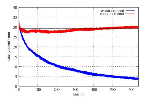
**Fig. 12.** Total water content of the Grenzhof soil sample, measured by TDR (blue), and the mass balance  $\eta\theta_I(t) + \int_0^t j_{\rm exp}^w(\tau) d\tau$  (red). The black horizontal line represents the initially measured water content.
