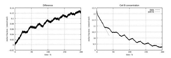
**Fig. 3.** Water vapour molar fraction measurements of the gas analyser with conditioned air at 10°C dew point flowing simultaneously through both cells of the instrument. The difference (left) is very stable while the absolute molar fraction (right) is drifting faster, with about  $-49 \mu$ mol mol<sup>-1</sup> h<sup>-1</sup> on the first day (dashed line).
