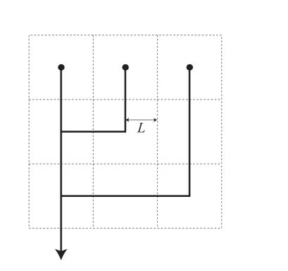
**Fig. 1.** Cartoon illustrating the relationship between hillslope length and drainage density. A tile with an area of  $A=4L^2$  has a channel length of (averaged over all tiles)  $\approx 2L$ , resulting in a drainage density of L/2.
