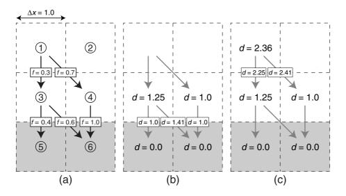
**Fig. 3.** Illustration of the multiple flow direction flow distance algorithm. (a): flow fractions *f* from every cell to at most 2 lower neighbours. (b): First step of d(c) computations. The small-print boxed number on top of the arrows indicate path lengths along that route. The large unboxed numbers in the cell centre indicate computed d(c) values. (c): Second and last step.
