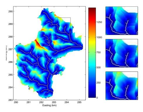
**Fig. 4.** Flow distance field for the Plynlimon catchments. Left: Flow distance as computed using the Quinn et al. (1991) flow fractionalisation method ("MFD-Q"). Right, top: detail showing the D8 single-flow direction method ("SFD"). Right, middle: detail showing the Tarboton (1997) multiple-flow-direction method ("MFD-T"). Right, bottom: detail showing the MFD-Q method.
