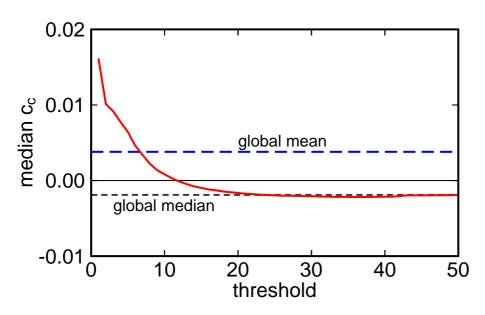
**Fig. 6.** Diagram illustrating the asymmetric tails of contour curvature distribution. For every threshold *i* the *i*th and the (100-i)th percentiles have been computed. The red solid line indicates the average of these two percentiles. The dashed lines indicate the global mean curvature (>0; convergent) and global median curvature (<0; divergent).
