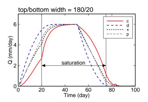
**Fig. 9.** Hydrological response for hillslopes with top/bottom widths of 20 and 1800 m (case II). Legends as for Fig. 8. The arrow marks the period during which saturation was obtained at the foot of the convergent hillslope.
