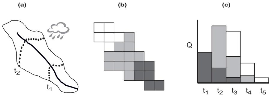
**Fig. 3.** Channel routing by a spatially distributed unit hydrograph approach: **(a)** a catchment can be divided into areas of isochrones; **(b)** isochrones are determined according to the mean travel time of channel water flows from a given cell to the catchment outlet; **(c)** unit hydrograph ordinates from individual isochrone areas are linearly superposed to estimate the total discharge.
