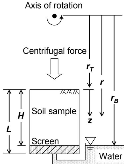
**Fig. 1.** Cross-sectional diagram of a soil sample in a centrifugal field, with free water establishing a hydrostatic pressure boundary condition at the bottom of the sample.
