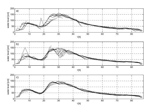
**Fig. 13.** DRI input data set – testing phase. Ensemble of the water levels forecasted at 1, 3 and 6 h ahead starting from each hour of the flood event considered. **(a)** FL-M model, **(b)** FL-TS model, **(c)** ANN model.
