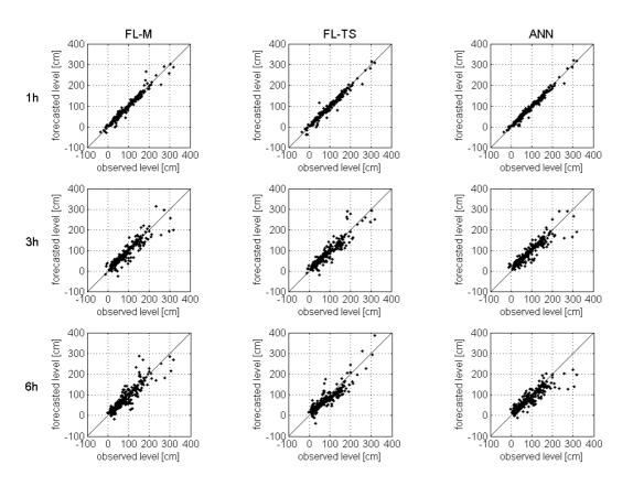
**Fig. 4.** ARI input data set – testing phase. Water levels forecasted at 1, 3 and 6 h ahead (rows 1, 2 and 3, respectively) by the FL-M, FL-TS and ANN models (columns 1, 2 and 3 respectively) versus the observed data.
