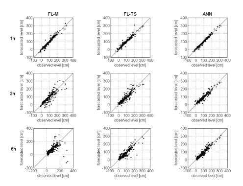
**Fig. 12.** DRI input data set – testing phase. Water levels forecasted at 1, 3 and 6 h ahead (rows 1, 2 and 3, respectively) by the FL-M, FL-TS and ANN models (columns 1, 2 and 3 respectively) versus the observed data.
