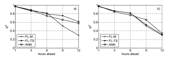
**Fig. 3.** ARI input data set.  $R^2$  relevant to FL-M, FL-TS and ANN models. **(a)** training phase, **(b)** testing phase.
