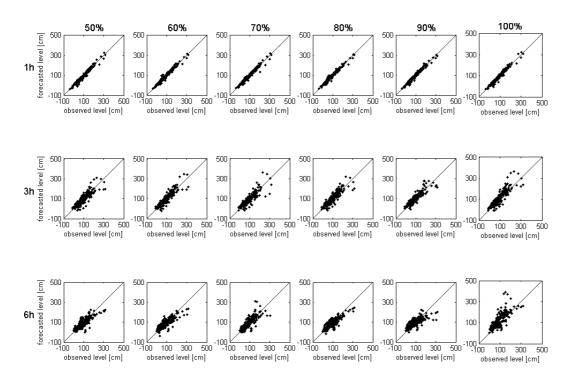
**Fig. 7.** ARI input data set – testing phase. Scatter plots of the water levels forecasted at 1, 3 and 6 h ahead (rows 1, 2 and 3 respectively) by the FL-M model trained with data set characterized by different percentage of positive water level variations (columns 1–6).
