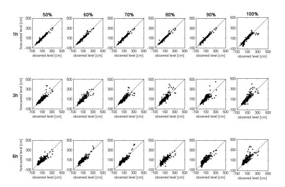
**Fig. 8.** ARI input data set – testing phase. Scatter plots of the water levels forecasted at 1, 3 and 6 h ahead (rows 1, 2 and 3 respectively) by the FL-TS model trained with data set characterized by different percentage of positive water level variations (columns 1–6).
