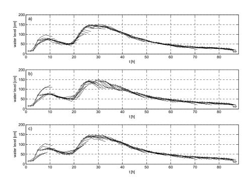
**Fig. 5.** ARI input data set – testing phase. Ensemble of the water levels forecasted at 1, 3 and 6 hours ahead starting from each hour of the flood event considered. **(a)** FL-M model, **(b)** FL-TS model, **(c)** ANN model.
