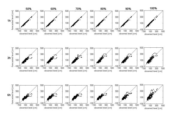
**Fig. 9.** ARI input data set – testing phase. Scatter plots of the water levels forecasted at 1, 3 and 6 h ahead (rows 1, 2 and 3 respectively) by the ANN model trained with data set characterized by different percentage of positive water level variations (columns 1–6).
