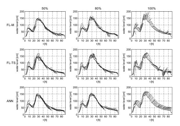
**Fig. 10.** Ensemble of the water levels forecasted at 1, 3 and 6 h ahead starting from each hour of the flood event considered by FL-M, FL-TS and ANN models (rows 1, 2 and 3 respectively) trained with data set characterized by different percentage of positive water level variations (columns 1–3).
