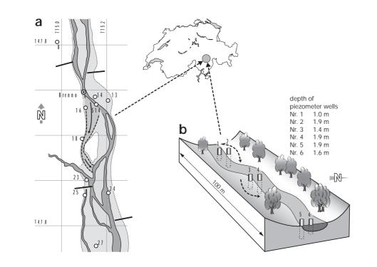
**Fig. 1.** Plan view of Valle di Blenio, Alps of Southern Switzerland. **(a)** Plan view of the first site: Circles: monitoring wells; dotted circles: logger in Brenno River; dashed line: flood bank; thin lines: bank structures; arrow: change of main river course by a flood. **(b)** Block diagram of the second site showing shallow monitoring wells; arrows: change of main river course by a flood.
