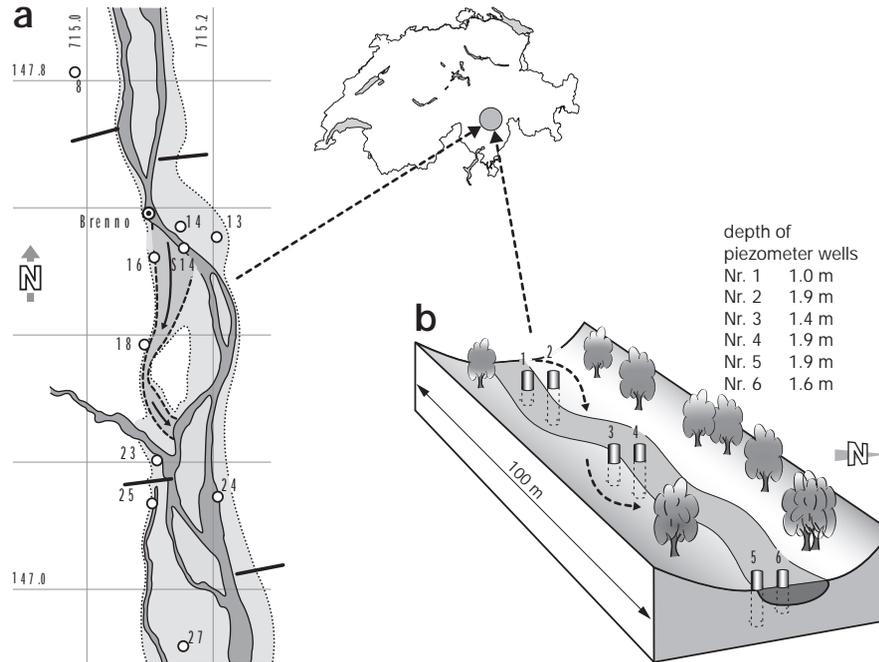
**Fig. 1.** Plan view of Valle di Blenio, Alps of Southern Switzerland. **(a)** Plan view of the first site: Circles: monitoring wells; dotted circles: logger in Brenno River; dashed line: flood bank; thin lines: bank structures; arrow: change of main river course by a flood. **(b)** Block diagram of the second site showing shallow monitoring wells; arrows: change of main river course by a flood.
