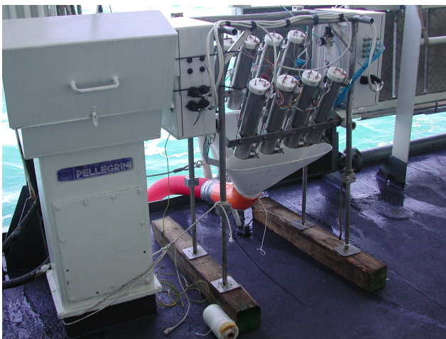
Fig. 4. The multiple launcher on the deck of the Italian Hydrographic Institute ship Magnaghi.
