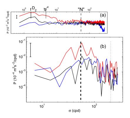
**Fig. 5.** *W*-spectra from summertime-INP ADCP-data at  $-22.5 \,\mathrm{m}$  (red) and  $-39.5 \,\mathrm{m}$  (black), in comparison with w at  $-22.5 \,\mathrm{m}$  inferred from temperature data using Eq. (1) (blue). (a) For entire 8-d period. (b) For period of Fig. 3b between days 194.70 and 194.85. The dashed line indicates the buoyancy frequency corresponding to a period of 1600 s ( $\sim$  bottom boundary layer) and the dotted line indicates a period of 420 s (lower pycnocline).
