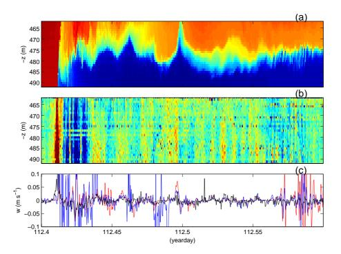
**Fig. 6.** W-test for frontal solibore in 5-h detail in FSC-data. **(a)** High-resolution temperature measured using NIOZ-1. Values between [2, 8]°C (blue–red). **(b)** Corresponding ADCP's w-data. Values between [-0.04, 004] m s $^{-1}$  (blue–red). **(c)** W at 477 m from ADCP (black) and inferred from temperature data using Eq. (1) and unsmoothed local vertical temperature gradient (blue), and time mean temperature gradient (red).
