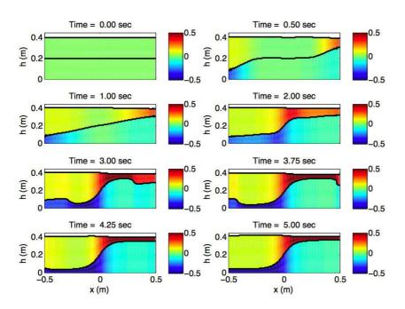
**Fig. 2.** Development of two layer flow (for a channel with  $b_{\text{max}}$ =0.3 m).
