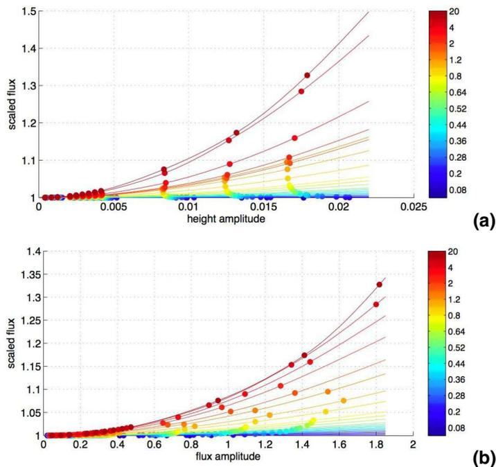
**Fig. 8.** Flux is plotted against (a) measured height amplitude and (b) measured flux amplitude, with  $\gamma$  in colour. Solid circles show the original points from which the other points have been interpolated.
