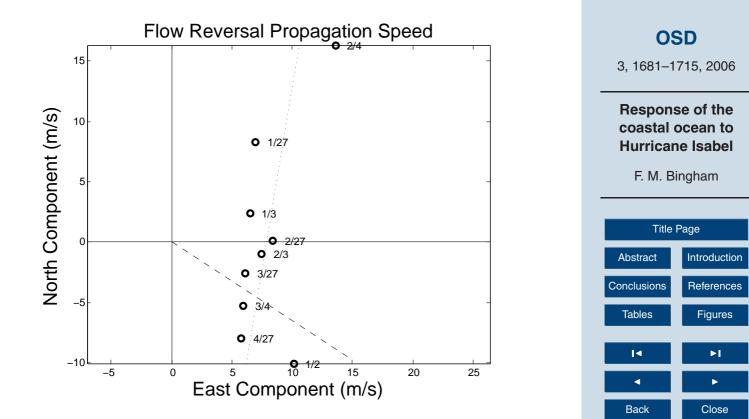
**Fig. 10.** Propagation of the flow reversal across the CORMP array. Individual points are labeled with the appropriate pair of moorings. For example, point labeled "1/27" shows the speed and direction of propagation of the flow reversal from OB1 to OB27. Dotted line is a least squares fit to the points shown. Dashed line points 33° below the x-axis, approximately the offshore direction.
