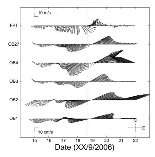
Fig. 8. Stick diagram of winds at FPT (top series) and low-pass currents at other moorings as shown at left. A scale for the winds is shown at the top left and for the currents at bottom left.
