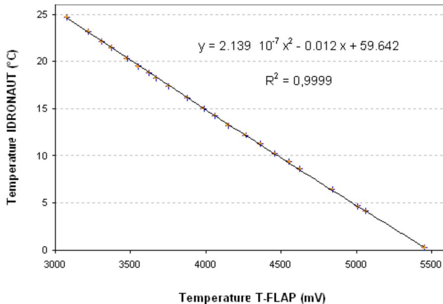
**Fig. 8.** On X axis there is the temperature measured by T-Flap (mV) while on Y there is the temperature measured by Idronaut expressed in °C.
