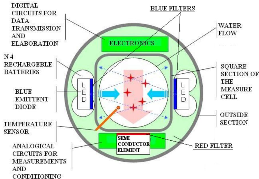
**Fig. 3.** A schematic section of the measurement cell.
