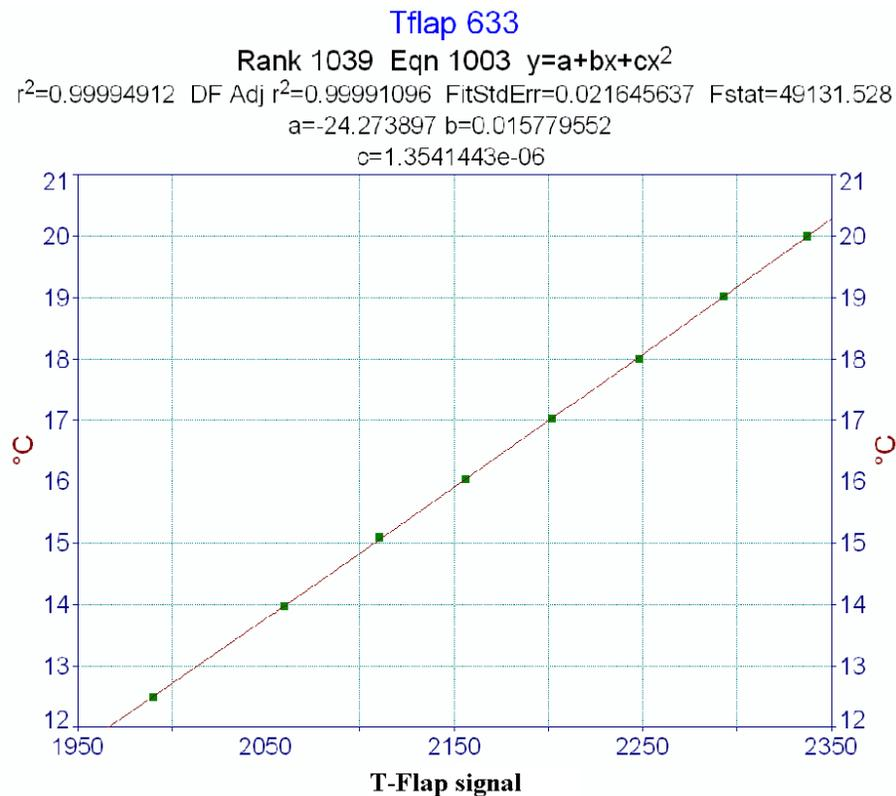
**Fig. 9.** Best Fit curve for the calibration of the temperature sensor: on Y is reported the temperature measured by OTM Falmouth (°C) and on X is reported the signal given by the T-Flap's temperature sensor.
