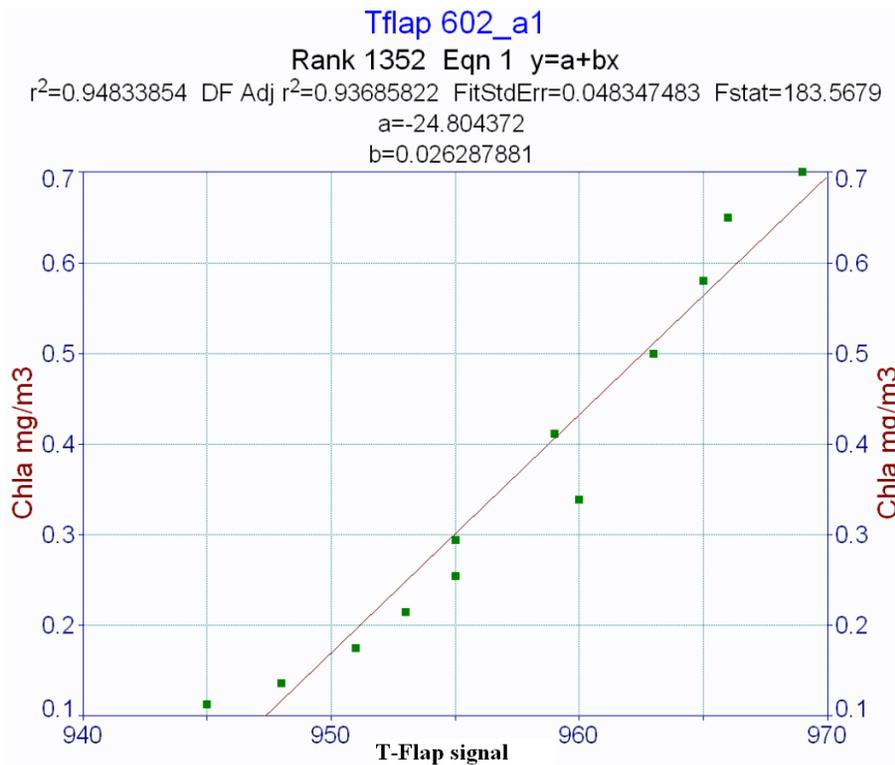
**Fig. 6.** On X axis there is the Chl “a” measured by T-Flap (mV) while on Y there is the Chl “a” measured by PrimProd 1.08 expressed in  $\text{mg}/\text{m}^3$ .
