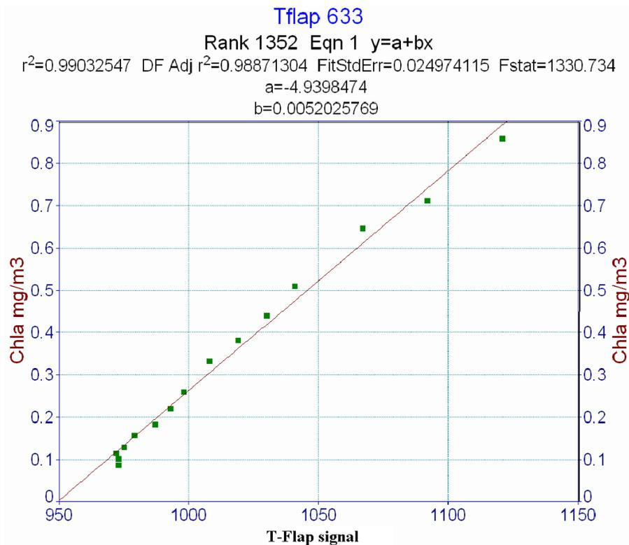
**Fig. 7.** Best Fit curve for the calibration of the T-Flap fluorescence sensor: on Y is reported the Chlorophyll concentration measured by PrimProd ( $\text{mg/m}^3$ ) and on X is reported the signal given by the T-Flap's fluorescence sensor.
