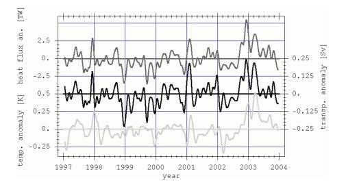
**Fig. 10.** Low-pass filtered (cut-off frequency:  $(30 \text{ days})^{-1}$ ) anomalies relating to the seasonal signals shown in Fig. 8. The uppermost, dark-grey curve shows the NIIC's simulated heat flux anomalies at section 7. The black curve in the middle shows the NIIC's volume flux anomalies normal to section 7. The light-grey curve below shows the spatially averaged water temperature over the North Icelandic shelf (area between section 7 and 12 with water depth below 300 m).
