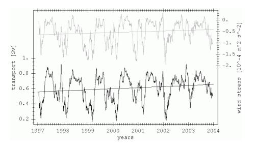
**Fig. 9.** 31 day moving averages of the northerly wind stress component (NCEP) (divided by the water density of 1030 kg m<sup>-3</sup>) at 67°40′ N, 22°32′W (upper curve) and simulated volume flux of the NIIC normal to section 7 (lower curve). Trends 1997–2003 are:  $3.2 \ 10^{-6} \ m^2 \ s^{-2}$  per year for the wind stress, and 0.014 Sv per year for the volume flux.
