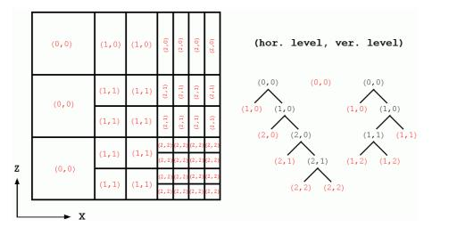
**Fig. 2.** Scheme of the computational mesh consisting of differently sized cells (left) and scheme of the mesh producing tree algorithm (right).
