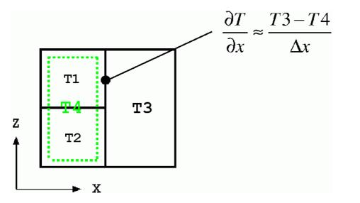
**Fig. 3.** The computational scheme for the horizontal gradient of temperature or salinity between grid cells of different thickness. Consider the horizontal homogenous but stratified case. I.e.  $0.5 \times (T1+T2)=T3$  and  $T1 \neq T2$ . In order to avoid the spurious gradient between T1 and T3 the gradient is computed between T3 and the parent cell of T1, the cell T4= $0.5 \times (T1+T2)$ . Hence the horizontal gradient is zero.
