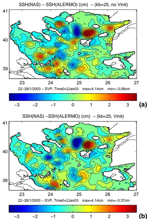
**Fig. 6.** Difference in the simulated sea surface height between the nested **(a)** NAS model (kb=25, no Vinit); **(b)** NAS model (kb=25, Vinit) and the outer ALERMO model: SSH(NAS)-SSH(ALERMO), averaged for 22–28 January.
