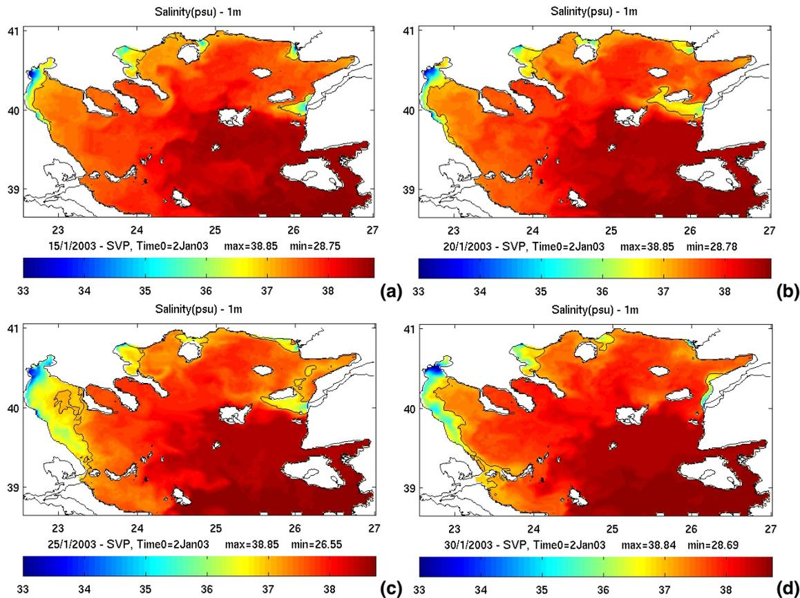
**Fig. 10.** Daily averaged, model simulated near surface salinity for N. Aegean on (a) 15 January 2003; (b) 20 January 2003; (c) 25 January 2003 and (d) 30 January 2003; the contour line marks the 37 isohaline.
