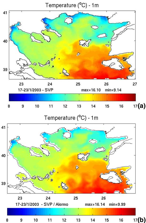
**Fig. 9.** Sea surface temperature weekly averaged for 17–23 January 2003 as simulated by (a) the N. Aegean model and (b) as simulated by the ALERMO model.
