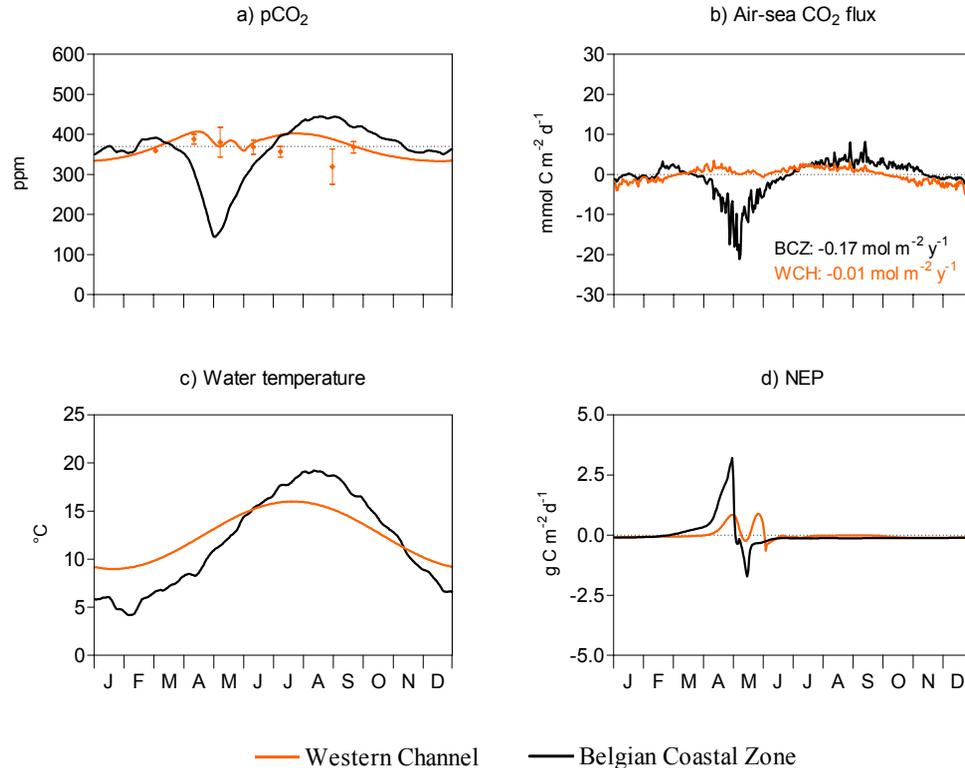
**Fig. 6.** Seasonal evolution of daily modelled (a) pCO<sub>2</sub>, (b) air-sea CO<sub>2</sub> flux, (c) water temperature and (d) net ecosystem production computed for WCH and BCZ boxes. Model results of pCO<sub>2</sub> in WCH (solid line) are compared with available observations in that area (◇). The dotted line, in the pCO<sub>2</sub> plots, corresponds to atmospheric pCO<sub>2</sub>. The calculated annual CO<sub>2</sub> air-sea flux is added to each plot of air-sea CO<sub>2</sub> flux.
