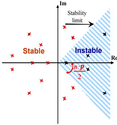
Fig. 7. Stability/instability area for a half-order system.
