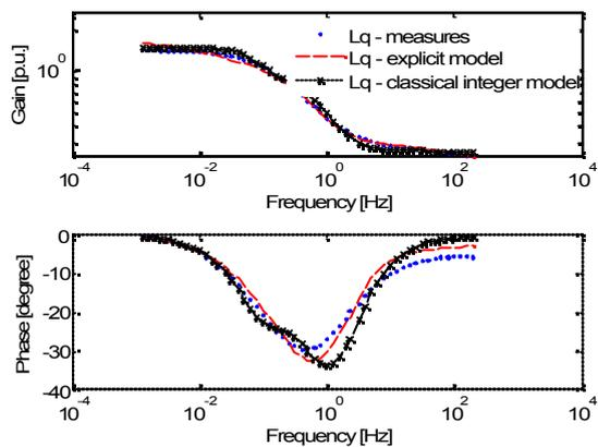
Fig. 8.b. Q-axis operational inductance identification.
