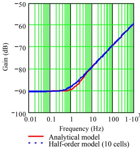
Fig. 3. Comparison between the analytical and half order approximation of the damper bar impedance.
