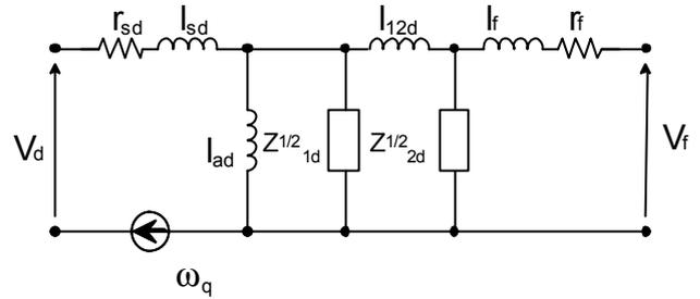
Fig. 4. Synchronous machine, direct axis equivalent half-order circuit
