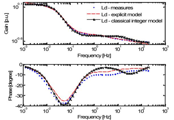
Fig. 8.a. D-axis operational inductance identification.
