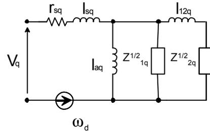
Fig. 5. Synchronous machine, quadrature axis equivalent half-order circuit
