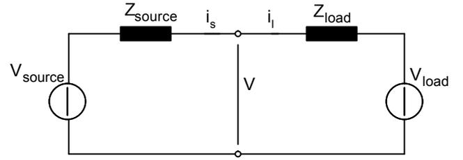
Fig. 6. Thevenin equivalent circuit of the studying system.
