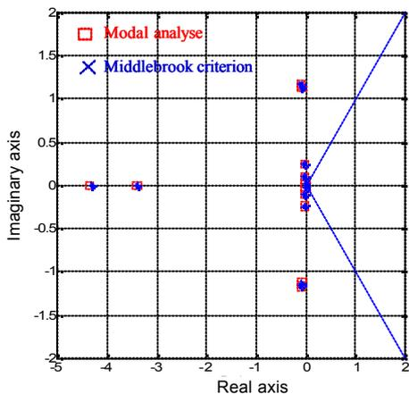
Fig. 9. System poles given by modal analysis and Thevenin-based impedance approach
