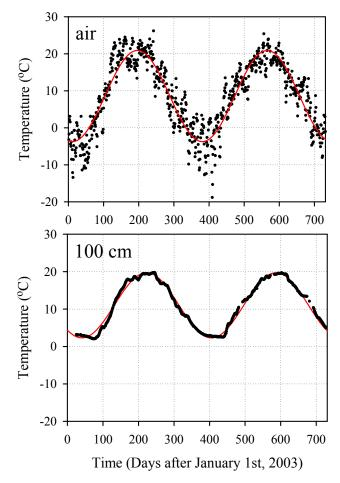
**Fig. 10.** Daily SAT and 100 cm soil temperatures recorded at Bistrita station for 2003 and 2004. The sinusoidal function fit is illustrated with red line.
