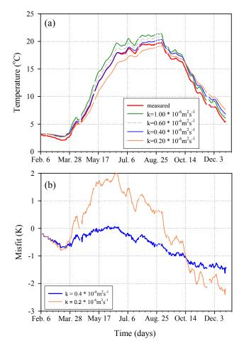
**Fig. 8. (a)** Heat transfer from 50 to 100 cm: measured and modelled daily 100 cm soil temperatures at Bistrita for 2003, using different values of thermal diffusivity for the 50–100 cm layer of soil. (b) The misfit between the measured and modelled temperatures for two thermal diffusivities:  $0.2 \times 10^{-6} \text{ m}^2 \text{ s}^{-1}$  and  $0.4 \times 10^{-6} \text{ m}^2 \text{ s}^{-1}$ .
