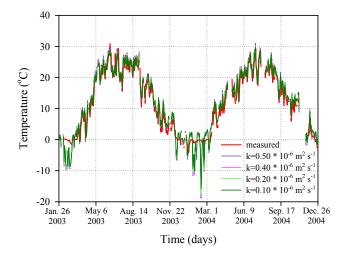
**Fig. 7.** Measured and modelled soil 5 cm temperature variations (daily averages) at Bistrita for 2003 and 2004, using different values of thermal diffusivity for the 0–5 cm layer of soil.
