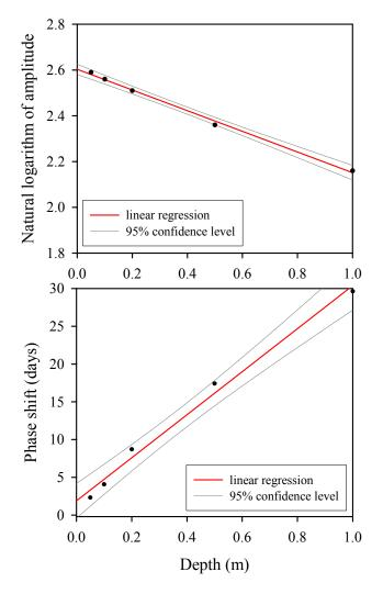
**Fig. 11.** Natural logarithm of amplitude and phase shift relative to the SAT as function of depth for Bistrița. The coefficient of determination of the regression line is  $r^2=0.996$  and  $r^2=0.990$  for amplitude and phase shift, respectively. The 95% confidence interval is also included.
