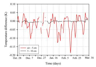
**Fig. 6.** Variation in time of the temperature differences for SAT-5 cm (red line) and for 5–10 cm (black line) layers, at Bistrița station for the winter season 2003–2004.
