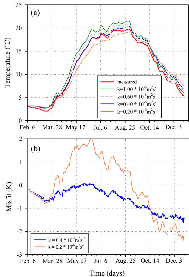
**Fig. 8.** (a) Heat transfer from 50 to 100 cm: measured and modelled daily 100 cm soil temperatures at Bistrița for 2003, using different values of thermal diffusivity for the 50–100 cm layer of soil. (b) The misfit between the measured and modelled temperatures for two thermal diffusivities:  $0.2 \times 10^{-6} \text{ m}^2 \text{ s}^{-1}$  and  $0.4 \times 10^{-6} \text{ m}^2 \text{ s}^{-1}$ .
