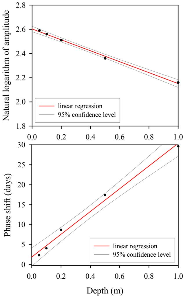
**Fig. 11.** Natural logarithm of amplitude and phase shift relative to the SAT as function of depth for Bistrița. The coefficient of determination of the regression line is  $r^2=0.996$  and  $r^2=0.990$  for amplitude and phase shift, respectively. The 95% confidence interval is also included.
