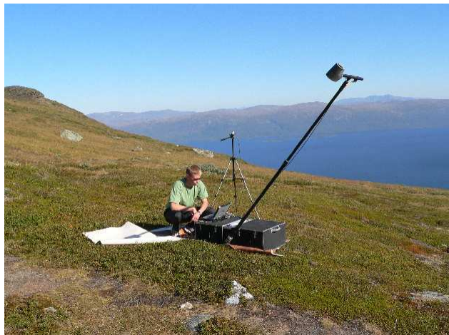
Fig. 2. Figifigo measuring BRF in Abisko, Sweden.
