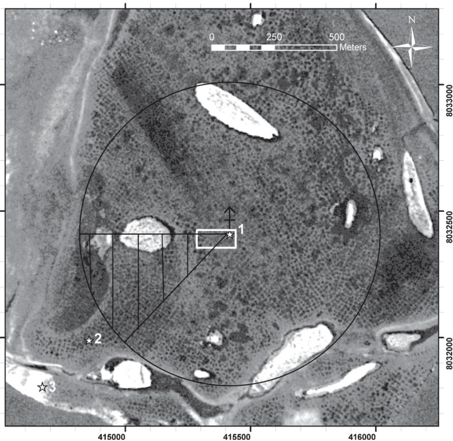
**Fig. 2.** CORONA satellite image of Samoylov Island, taken on 22 June 1964. The star symbols mark the position of (1) the eddy covariance system, (2) the long-term meteorological and soil station, and (3) the field laboratory. The black circle marks the 600 m radius around the eddy tower, and the hatched area marks the sector of discarded data due to disturbance from the power generator.
