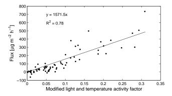
**Fig. 5.** Measured isoprene flux versus light and temperature activity factor  $(C_L C_T)$ . Linear fit of the dataset determines the standard emission potential. Lower panel show the results of the modified model described in the text.
