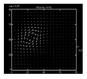
Fig. 2. Horizontal velocity used as boundary condition of the model to approximate the velocity pattern obtained in Fig.1.
