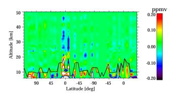
**Fig. 4.** Difference between retrieval with cloud-threshold 4.0 and 1.8 (RET\_A+AB\_MIPAS). The red and black curves show the lowermost tangent heights taken into account for retrieval after application of cloud-threshold 1.8 and 4.0, respectively.
