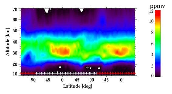
**Fig. 1.** Reference ozone distribution (RET\_A+AB\_MIPAS, data version V2\_O3\_2), derived from MIPAS limb-scans along orbit 8597 of 22 October 2003, 16:15-17:53 UT, plotted versus geographic latitude and altitude. Plus signs indicate the latitudinal locations of the limb-scans on the daytime (white signs) and nighttime part (red signs) of the orbit; the small white areas indicate retrieved volume mixing ratios below 0 ppmv (due to profile oscillations).
