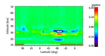
**Fig. 8.** Difference between retrieval with assignment of a common continuum background emission profile to adjacent microwindows within a 5 cm<sup>-1</sup> spectral range and retrieval with individual continuum profiles for every microwindow (RET\_A+AB\_MIPAS). Same meaning of plus signs as in Fig. 1.
