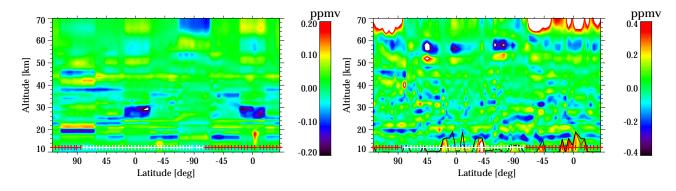
Fig. 10. Left: Difference between  $O_3$  retrieval with zero a-priori profile and reference retrieval (RET\_A+AB\_MIPAS). Right: Difference between retrieval with zero a-priori and reduced regularization strength and reference retrieval. Same meaning of plus signs as in Fig. 1.
