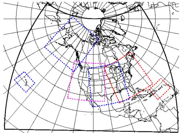
**Fig. 2.** Domains of the Eta 12 km operational model during the time of the scores shown in Figs. 3–5, February 2004–January 2005, heavy black line, and of the “high resolution windows” of the nested NMM model (Nonhydrostatic Mesoscale Model), dashed color lines. (Plot courtesy of Eric Rogers).
