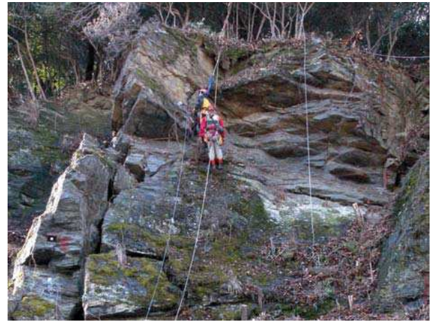
Fig. 3. A rock-climber installing vibrometers.
