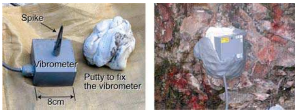
Fig. 2. Vibrometer shape and its installation.
