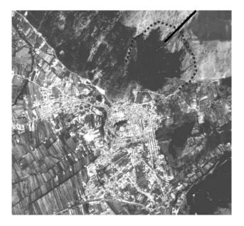
**Fig. 1.** Aerial photograph of Celano town: are indicated the landslide failure surface (dashed line) and the S. Vittorino fault (solid line).
