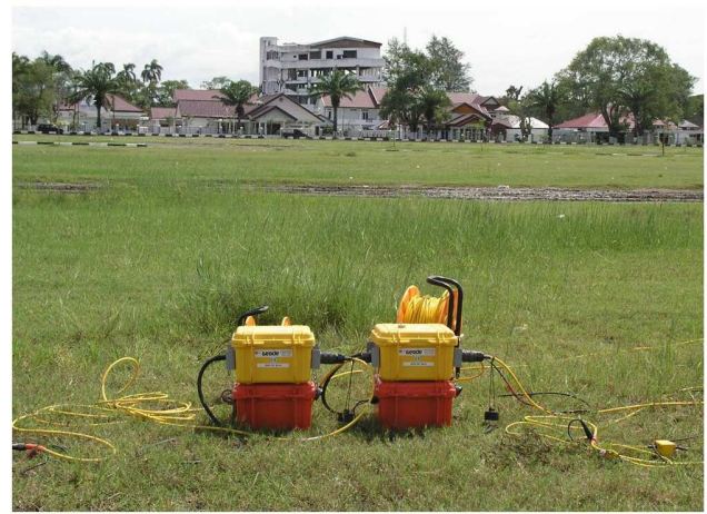
Fig. 2. Shallow shear-wave site investigation at Blang Padang place, centre of Banda Aceh city. Foreground: 48 channel Geode system used for seismic data acquisition. Centre: Local mud zone indicating local subsidence of young sediments. Background: Houses of nearly traditional Indonesian building style that were only slightly affected by earthquake shakings. In contrast, the high concrete building (demolition in 2006) shows severe structural damages and partly total collapse due to the earthquake shaking of 26 Dec 2004.
