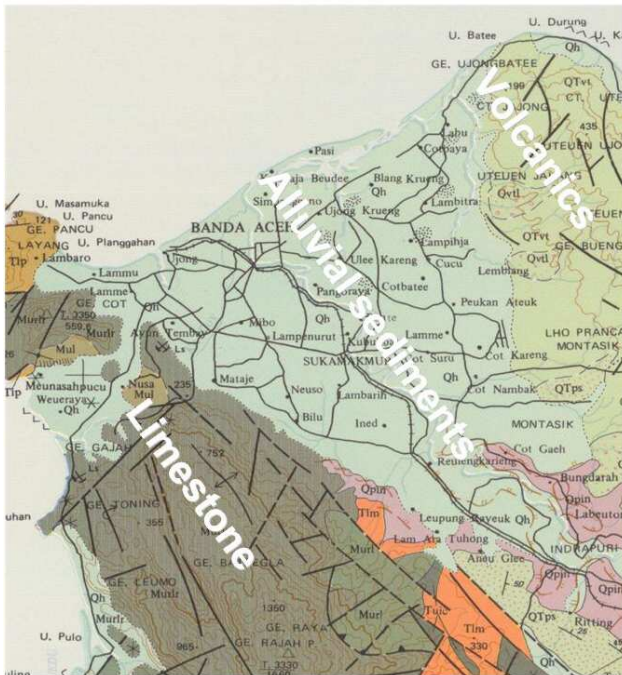
Fig. 1. Scene of the geologic map (Bennett et al., 1981) of the Krueng Aceh River delta showing undifferentiated alluvial sediments in the whole investigation area, adjacent to volcanic rocks (NE) and limestones (SW). Post tsunami ground-water exploration drilling in the alluvial delta has yielded stacks of organic clay, silt, sand, and gravel down to a depth of 220 m.
