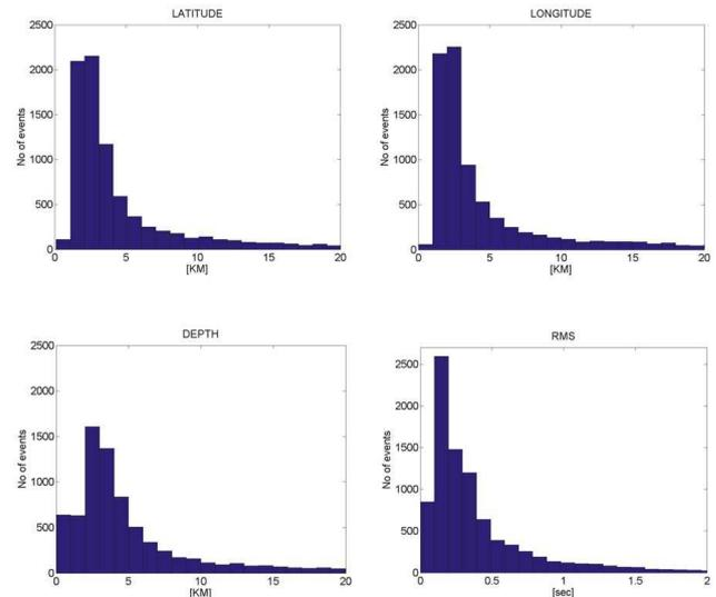
**Fig. 2.** Error distribution for events of the Izmit aftershock hypocenter catalog as determined from the combined GTF and SABONET network. The error is given in kilometer for latitude, longitude and depth, respectively, and in seconds for the root mean square (RMS) value. Approximately 70% percent of all events have a location error better than 5 km in all three directions and a RMS better than 0.3 s.
