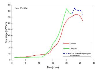
Fig. 6. Four-hour flood forecasting using the Philip's method.
