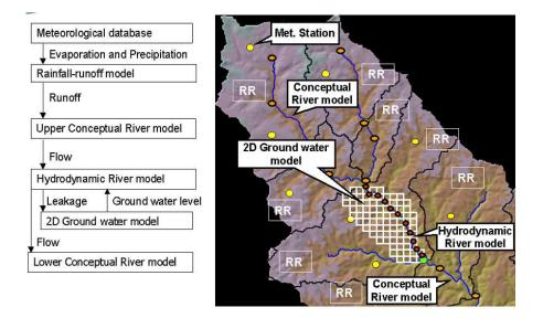
Fig. 1. Example of integrated catchment modelling that can be realised by combining OpenMI compliant models.
