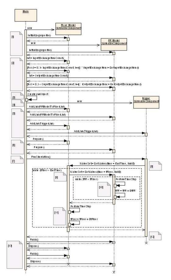
Fig. 6. Sequence diagram for OpenMI configuration with a Rainfall-runoff model linked to a river model.
