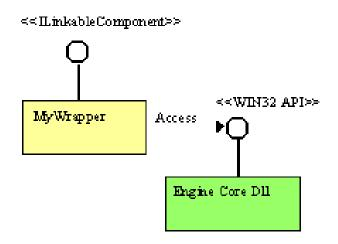
Fig. 7. Model engine wrapping design pattern.
