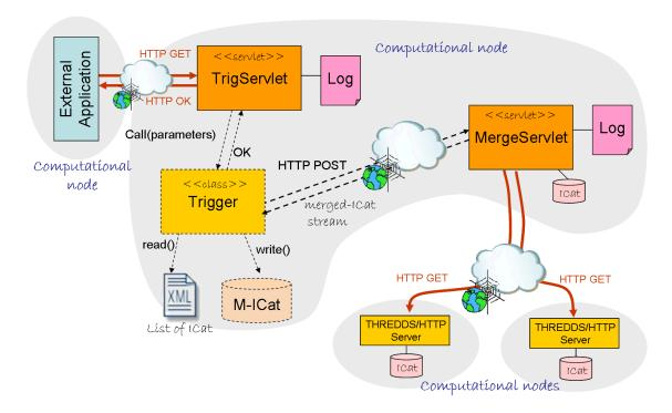
Fig. 6. Synchronization and merging use-case basing on the Trigger Service.
