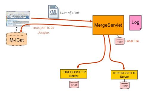
Fig. 4. TDM Collaboration/Deployment diagram.
