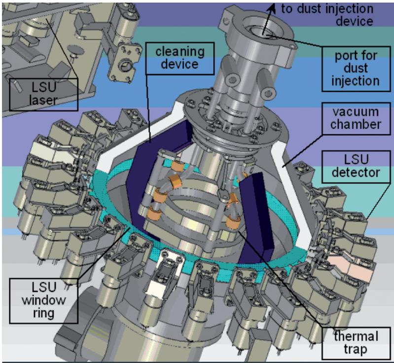
◀ FIG. 3: Sketch of the design of the new instrument for Columbus with its crown of detectors of the Light Scattering Unit (LSU). The inner diameter of the chamber (light blue ring) is about 10 cm (courtesy of Verhaert Space).
