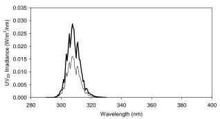
**Fig. 1.** Diffuse (light line) and global (heavy line) spectral UV irradiances taken on 17 August 2005 at approximately 11:00 EST and the spectral ratio of diffuse to global UV (a); and global and diffuse spectral irradiances from Fig. 1a weighted with the pre-vitamin  $D_3$  action spectrum (CIE, 2006) (b).
