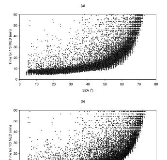
**Fig. 2.** The times required for an exposure of 1/3 MED due to diffuse  $UV_{ery}$  (**a**) and global  $UV_{ery}$  (**b**) as a function of SZA for all sky conditions during 2003.
