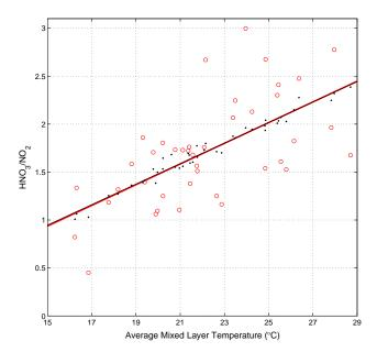
**Fig. 5.** HNO<sub>3</sub>/NO<sub>2</sub> shown as single daily averages (medians) during hours 12–16 vs. average mixed layer temperature. Observations (red circles), modeled values (black points), and the coincident best fit lines are shown.
