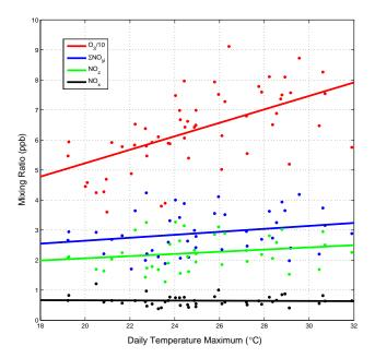
**Fig. 4.**  $O_3$ ,  $\Sigma NO_{yi}$ ,  $NO_z$ , and  $NO_x$  shown as single daily averages (medians) during hours 12-16 vs. daily temperature maximum. Best fit lines shown have parameters (from top to bottom): slopes=2.24, 0.049, 0.036, -0.0007 °C<sup>-1</sup> and  $R^2$  values=0.43, 0.052, 0.043, 0.002.
