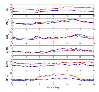
**Fig. 2.** Diurnal cycles of  $O_3$ ,  $\Sigma NO_{yi}$ ,  $NO_x$ ,  $\Sigma PNs$ ,  $\Sigma ANs$ , and  $HNO_3$  shown for half-hour intervals of the 17th and 83rd percentile of the measurements as ordered by the associated daily temperature maximum ( $T_{max}$ );  $T_{max}$  17th percentile=20.8°C (blue),  $T_{max}$  83rd percentile=28.4°C (red).
