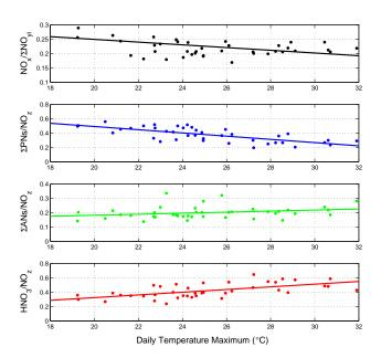
**Fig. 3.**  $NO_x/\Sigma NO_{yi}$   $\Sigma PNs/NO_z$ ,  $\Sigma ANs/NO_z$ , and  $HNO_3/NO_z$  shown as single daily averages (medians) during hours 12–16 vs. daily temperature maximum. Best fit lines shown have parameters (from top to bottom): slopes=-0.0048, -0.023, 0.0036, 0.019  $^{\circ}C^{-1}$  and  $R^2$  values=0.14, 0.52, 0.069, and 0.37.
