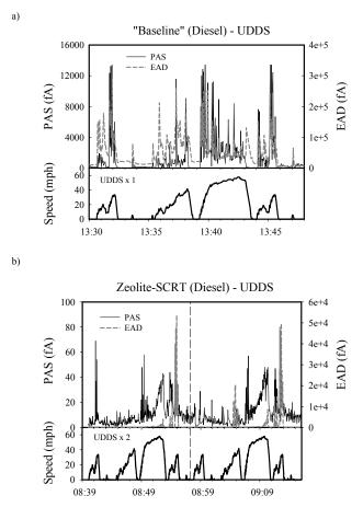
**Fig. 2.** Time series of the PAS and EAD signals (fA) for the "baseline" (a) and the Zeolite-based SCRT (b) vehicles, both operating in UDDS mode. Speed profiles during typical UDDS cycles are also reported.
