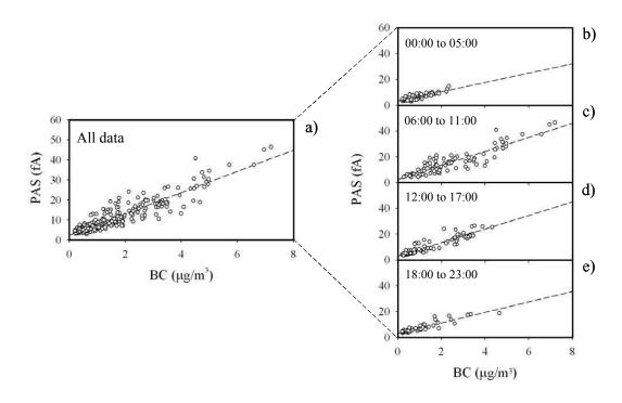
**Fig. 4.** PAS vs BC plots considering all measurements obtained at the Wilmington site in May 2007 (a), and the corresponding timesegregated data (b to e). Regression equations and correlation coefficients ( $R^2$ ) were: (a) y=5.31×+2.48,  $R^2$ =0.86; (b) y=3.62×+3.23,  $R^2$ =0.69; (c) y=5.44×+2.52,  $R^2$ =0.82; (d) y=5.27×+2.99;  $R^2$ =0.86; (e) y=4.04×+3.29,  $R^2$ =0.84.
