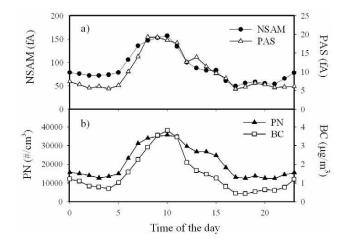
**Fig. 1.** Average hourly diurnal profiles of the photoelectric aerosol sensor (PAS) and nano-particle surface area monitor (NSAM) signals (**a**), and of the black carbon (BC) and particle number (PN) concentrations (**b**) measured at the Wilmington site in May 2007.
