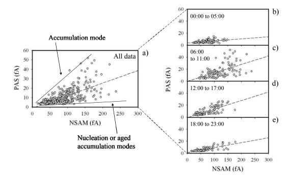
Fig. 3. PAS vs NSAM plots considering all measurements obtained at the Wilmington site in May 2007 (a), and the corresponding time-segregated data (b to e). Regression equations and correlation coefficients ( $R^2$ ) were: (a) y=0.13×-1.03,  $R^2$ =0.47; (b) y=0.04×+3.69,  $R^2$ =0.21; (c) y=0.14×-0.18,  $R^2$ =0.31; (d) y=0.14×-0.59;  $R^2$ =0.57; (e) y=0.08×+1.14,  $R^2$ =0.60.
