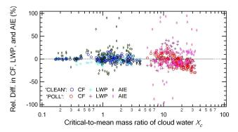
**Fig. 2.** The relative differences (Rel. Diff.) between the base cases ( $\varepsilon$ =0) and the sensitivity tests ( $\varepsilon$ =300) vs. the critical-to-mean mass ratio of cloud water ( $x_c$ ) averaged over all cloudy cells at the same model time for the "CLEAN" and "POLL" cases. The circle, plus, and diamond denote the instantaneous cloud fraction (CF), liquid water path (LWP), and aerosol indirect effect (AIE), respectively.
