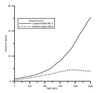
**Fig. 2.** Average time evolution for 1000 simulations versus time  $(N_0=100)$  of the largest and second largest droplets for the kernel Cxy ( $C=5.49\times10^{10}$  cm<sup>3</sup> g<sup>-2</sup> s<sup>-1</sup>).
