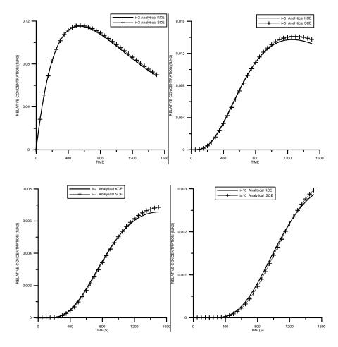
**Fig. 10.** Time evolution (bin sizes 2,5,7 and 10) for a system modeled by the sum kernel, as a function of time. The solid lines are the analytical solution of the KCE, the symbols are the analytical solutions of the SCE.
