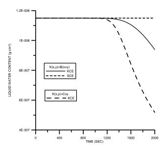
**Fig. 12.** Time evolution of the liquid water content (first moment of the distribution) for the sum kernel (K(x, y) = B(x + y)), calculated from size distributions of the KCE and true averages from the SCE, and for product kernel (K(x, y) = Cxy), calculated from the analytical solution of the KCE.
