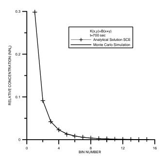
**Fig. 1.** The number of particles, averaged over 1000 simulations and normalized to initial number of particles ( $N_0$ =100), versus the analytical solution of the stochastic collection equation (SCE) at t=700 s, as a function of size.
