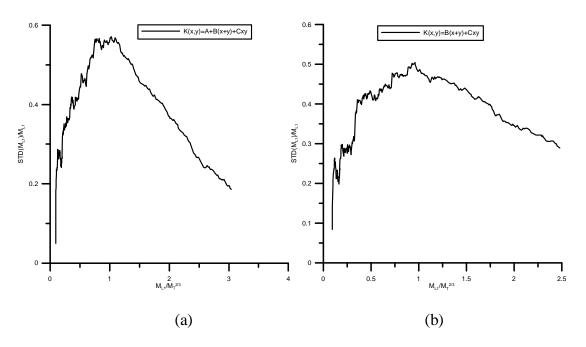
**Fig. 9.** The ratio of the standard deviation to expectation value of the largest droplet  $STD(M_{L1})/M_{L1}$  as a function of  $M_{L1}/M_T^{2/3}$  for approximating polynomials (a) A+B(x+y)+Cxy and (b) B(x+y)+Cxy.
