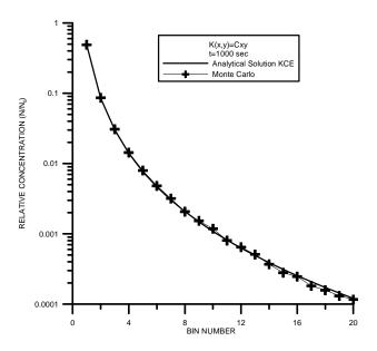
**Fig. 6.** Size distributions obtained from the KCE and the stochastic approach at t=1000 s for the product kernel.
