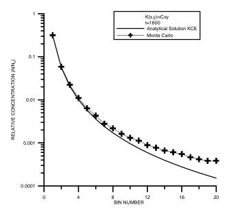
**Fig. 7.** Size distributions obtained from the KCE and the stochastic approach at t=1600 s for the product kernel.
