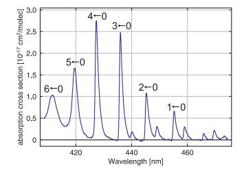
**Fig. 1.** Absorption cross section spectrum of iodine monoxide (Spietz et al., 2005) with an original FWHM of 0.07 nm, convoluted with the SCIAMACHY slit function. Eight excitation bands (six of them shown in the graph) from the ground state to the first excited state with different vibrational levels  $(A_{3/2}^2 \leftarrow X_{3/2}^2)$  can be identified, resulting in a very strong differential structure.
