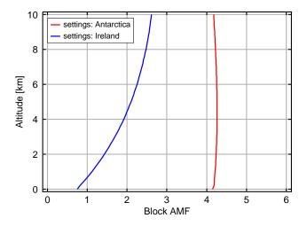
**Fig. 2.** Block air mass factors calculated with SCIATRAN Version 2.0 (Rozanov et al., 2005) for 425 nm, and two different example locations, red: 90% albedo,  $70^{\circ}$  solar zenith angle (typical for Antarctica, October 2005), blue: 5% albedo, 55° solar zenith angle (typical for Ireland). For the boundary layer, the AMF and with this the sensitivity for IO detection is several times higher for Antarctic conditions.
