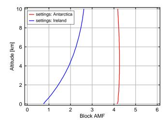
**Fig. 2.** Block air mass factors calculated with SCIATRAN Version 2.0 (Rozanov et al., 2005) for 425 nm, and two different example locations, red: 90% albedo, 70° solar zenith angle (typical for Antarctica, October 2005), blue: 5% albedo, 55° solar zenith angle (typical for Ireland). For the boundary layer, the AMF and with this the sensitivity for IO detection is several times higher for Antarctic conditions.
