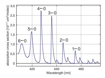
**Fig. 1.** Absorption cross section spectrum of iodine monoxide (Spietz et al., 2005) with an original FWHM of 0.07 nm, convoluted with the SCIAMACHY slit function. Eight excitation bands (six of them shown in the graph) from the ground state to the first excited state with different vibrational levels  $(A_{3/2}^2 \leftarrow X_{3/2}^2)$  can be identified, resulting in a very strong differential structure.
