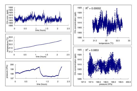
Fig. 3. Results of the laboratory experiment on the effect of  $T_{cell}$  and  $P_{cell}$  on CH<sub>4</sub> concentration measurements. (a) time series of CH<sub>4</sub> concentration measurements; (b) time series of  $T_{cell}$  measurements; (c) time series of  $P_{cell}$  measurements; (d) scatter plot of CH<sub>4</sub> concentration against  $T_{cell}$  with correlation coefficient ( $R^2$ ); (e) scatter plot of CH<sub>4</sub> concentration against  $P_{cell}$  with  $R^2$ .
