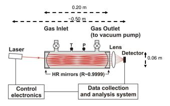
**Fig. 1.** Schematic overview of the integrated cavity output analysis (ICOS) technique used in the FMA. (Source: Los Gatos Research Ltd.) "*R*" is the reflectivity of the mirrors and "*T*" and "*P*" are the sensors of  $T_{cell}$  and  $P_{cell}$ .
