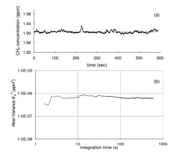
**Fig. 2.** Time series of  $CH_4$  concentration measurements with 10 Hz sampling rate with a mean of 1905 ppb and a standard deviation of 4.74 ppb (a) and the Allan variance plot for these data (b).
