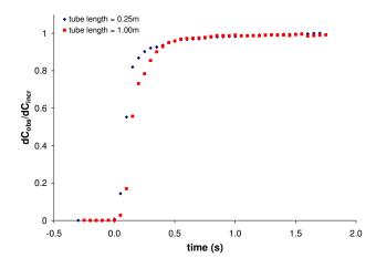
Fig. 5. Averaged and normalised time series of  $CH_4$  concentration data showing the instrument response with 20 Hz sampling rate changing from ambient air to a gas sample with a high  $CH_4$  concentration for tube lengths of 0.25 m and 1.0 m.
