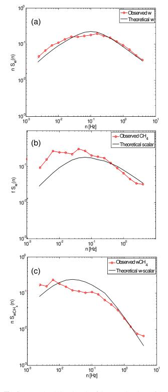
**Fig. 6.** Averaged and binned results of the spectral analyses of the FMA eddy covariance set-up for two moderately turbulent days (six half hour periods per day). (a) Observed and theoretical power-spectrum w; (b) Observed and theoretical power-spectrum of [CH<sub>4</sub>]; (c) Observed and theoretical co-spectrum of w'[CH<sub>4</sub>]<sup>'</sup>.
