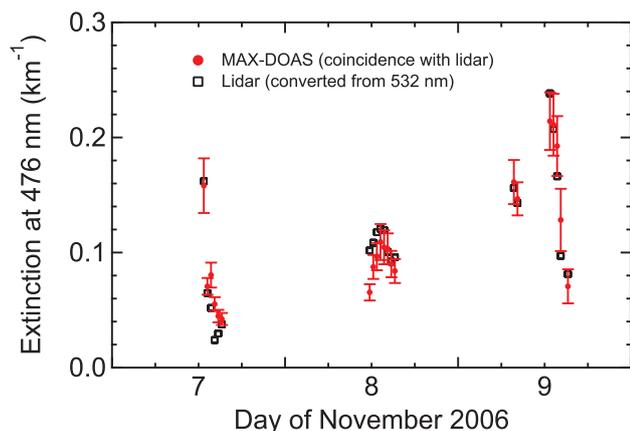
**Fig. 8.** Same as Fig. 7, but for the comparisons only for 7–9 November 2006. 6 November is omitted, because of no coincident measurements. Error bars represent errors estimated from the retrieval covariance matrix.
