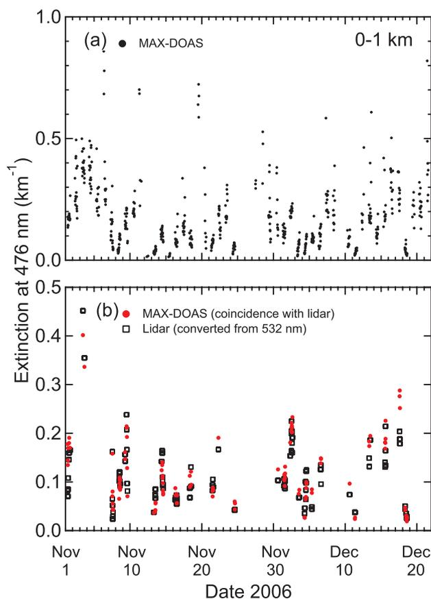
**Fig. 7.** (a) Time series of all the MAX-DOAS aerosol extinction coefficient ( $k$ ) data at 476 nm for the layer from 0 to 1 km. (b) Only coincident MAX-DOAS (red) and lidar (black) data are shown. Original lidar data have been converted to the values at 476 nm using the Ångström exponent derived from sky radiometer data.
