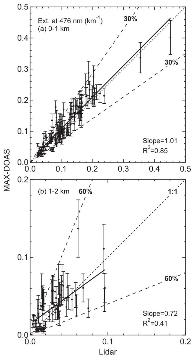
**Fig. 9.** Correlations between  $k$  values from MAX-DOAS and lidar for layers of (a) 0–1 and (b) 1–2 km. The 1:1 relationship and the 30% range are represented by the dotted line and dashed lines, respectively. Error bars represent errors estimated from the retrieval covariance matrix.
