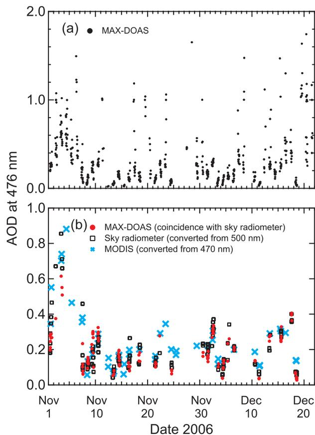
**Fig. 10.** (a) Time series of all the MAX-DOAS  $\tau$  (AOD) data at 476 nm. (b) Only coincident MAX-DOAS (red) and sky radiometer (black) data are shown. For reference, MODIS  $\tau$  data (sky blue) are also plotted. The original sky radiometer and MODIS data have been converted to the values at 476 nm using the Ångström exponent.
