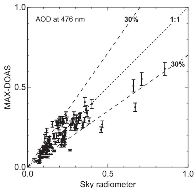
**Fig. 12.** Same as Fig. 9, but for the correlations between  $\tau$  (AOD) values at 476 nm from MAX-DOAS and sky radiometer data. Error bars represent the errors estimated from the retrieval covariance matrix.
