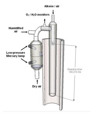
**Fig. 4.** Schematic of the calibrator based on the steady-state  $O_3$ -alkene technique.
