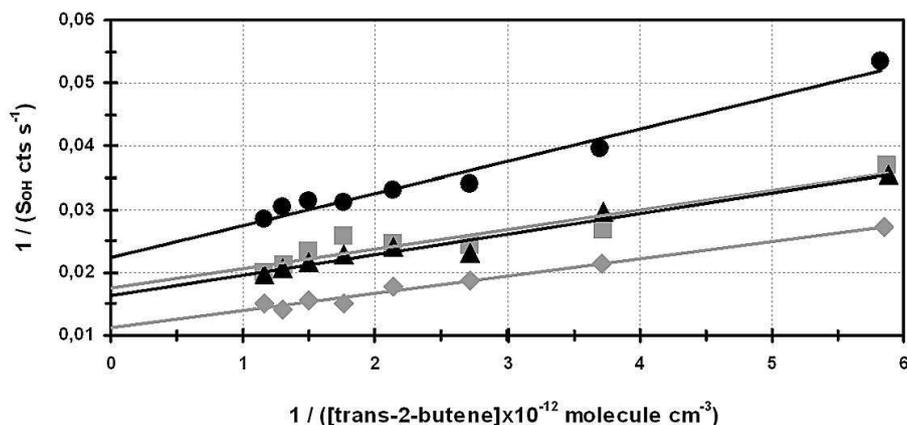
**Fig. 9.** Plot of  $1/S_{\text{OH}}$  versus  $1/[\text{trans-2-butene}]$  for 4 independent calibrations at various  $[\text{O}_3]$ ,  $[\text{water}]$  and laser power: Black circles 2.1 ppm  $\text{O}_3$ , 0.75% water, 1.0 mW; grey squares 2.2 ppm  $\text{O}_3$ , 0.47% water, 1.0 mW; black triangles 2.5 ppm  $\text{O}_3$ , 0% water, 0.9 mW; grey diamonds 2.4 ppm  $\text{O}_3$ , 0% water, 1.4 mW.
