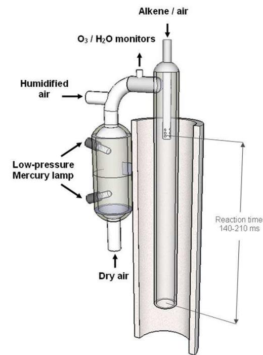
**Fig. 4.** Schematic of the calibrator based on the steady-state O<sub>3</sub>-alkene technique.
