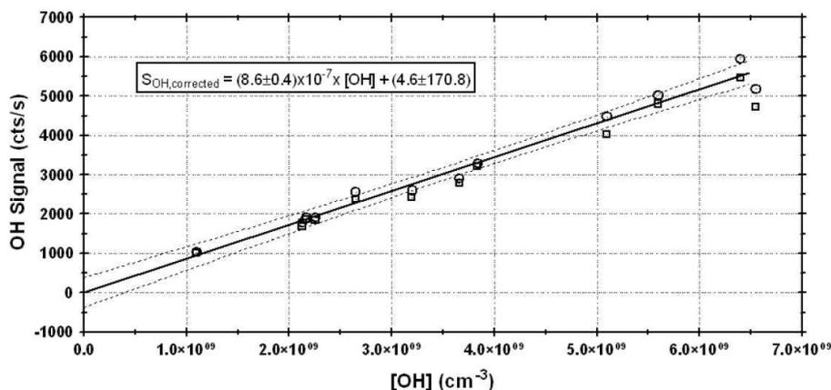
**Fig. 6.** Plot of  $S_{\text{OH}}$  versus  $[\text{OH}]$ . Open circles represent the OH signal corrected from the water-vapor quenching effect. Open squares represent the uncorrected signal. The dashed lines are the 95% confidence intervals of the linear regression for the corrected signal. The slope of the linear regression is a determination of  $R_{\text{OH}}$  under dry air conditions.
