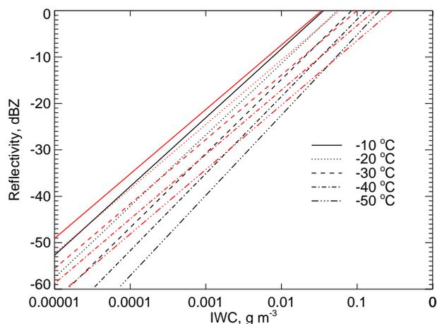
**Fig. 7.** Derivation of ice water content from cloud radar reflectivity by relations of IWC and dBZ according to Hogan et al. (2006), stratified by temperature, black lines: “best expected value”, red lines: “best variance”.
