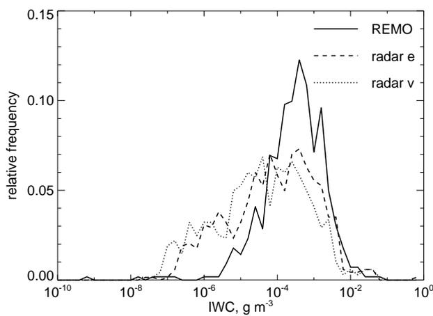
**Fig. 20.** Probability density functions of IWC derived from REMO and from cloud radar (using the algorithm of Hogan et al. (2006)) in the range of 6000 m to 10 000 m. The abbreviations “e” and “v” stand for the  $Z$ -IWC – algorithms optimizing the expected value and the variance of IWC, respectively.
