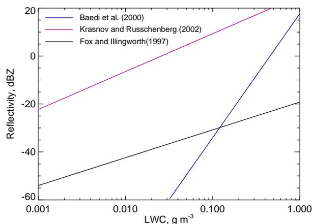
**Fig. 6.** Derivation of liquid cloud water content from cloud radar reflectivity by relations of LWC and dBZ from different authors, applied at different ranges of dBZ.
