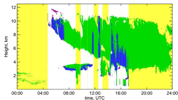
**Fig. 5.** Cloud mask derived from radar and lidar on 4 June 2004. Meaning of colors: yellow: no lidar observation, green: radar cloud, blue: radar and lidar cloud, purple: lidar cloud.
