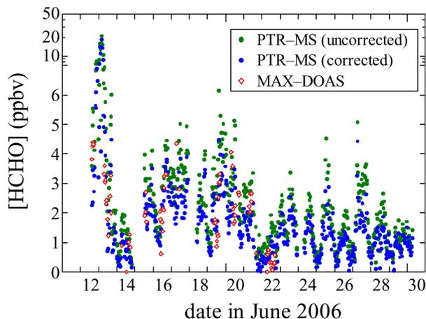
**Fig. 5.** Time variation of HCHO mixing ratios measured by PTR-MS and MAX-DOAS during a 19-day field campaign at Mount Tai in China. Uncorrected PTR-MS data points represent HCHO mixing ratios calculated from uncorrected M31 signals; corrected PTR-MS data points were calculated from M31 signals from which fragment ion signals at  $m/z$  31 from methyl hydroperoxide and alcohols (methanol and ethanol) were subtracted.
