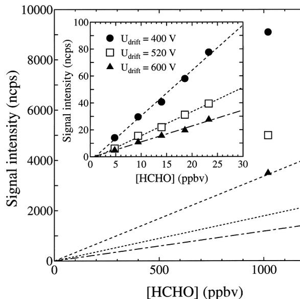
**Fig. 3.** Plots of normalized PTR-MS signal intensities at  $m/z$  31 vs. the HCHO concentrations at three drift tube  $E/N$  ratios in dry conditions. Inset: data obtained from the dynamic dilution method, with least-squares fit lines. Main figure: data obtained from the direct introduction method, with fit lines extrapolated from the dynamic dilution method.
