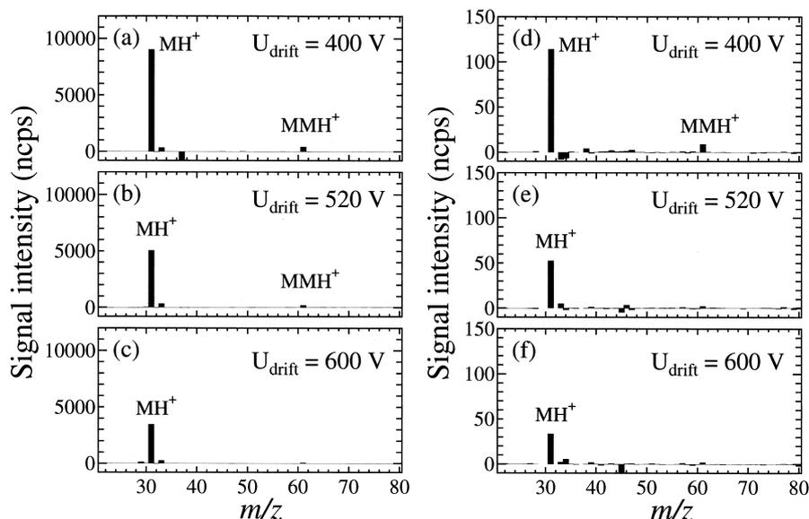
**Fig. 2.** Mass spectrum of HCHO at three different drift tube  $E/N$  ratios in dry conditions, obtained by the direct introduction method (a–c) and dynamic dilution method (d–f). (a–c):  $[\text{HCHO}] = 1.02$  ppmv; (d–f):  $[\text{HCHO}] = 23.3$  ppbv. Signals were normalized to a  $\text{H}_3\text{O}^+$  intensity of  $10^6$  cps, and background mass spectra without HCHO (obtained from  $\text{N}_2$  (a–c) or zero air (d–f) only) were subtracted.
