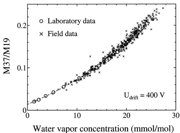
**Fig. 1.** Relative intensity of  $\text{H}_3\text{O}^+\cdot\text{H}_2\text{O}$  to  $\text{H}_3\text{O}^+$  (M37/M19) as a function of water vapor concentration (mmol/mol) in sample air. A dashed line shows the best-fit curve for data obtained in the laboratory.
