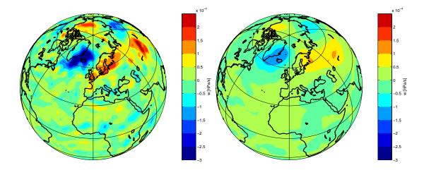
**Fig. 1.** Vertical wind from ERA-40 reanalysis data on standard pressure levels, calculated with two different methods. Left panel: Vertical wind field at 50 hPa from the continuity equation as provided by ECMWF, averaged over 1 January 2000 00:00–24:00 h (UTC) (to compare better with the right panel). Right panel: Vertical wind field from the thermodynamic equation and the Semi-Lagrangian approach for the staggered level between 30 and 50 hPa and 1 January 12:00 h (UTC).
